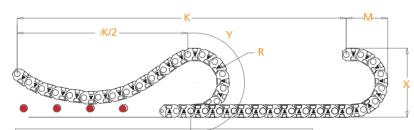
Should be used with supporting tray and rollers. Code of support roller is ST01
